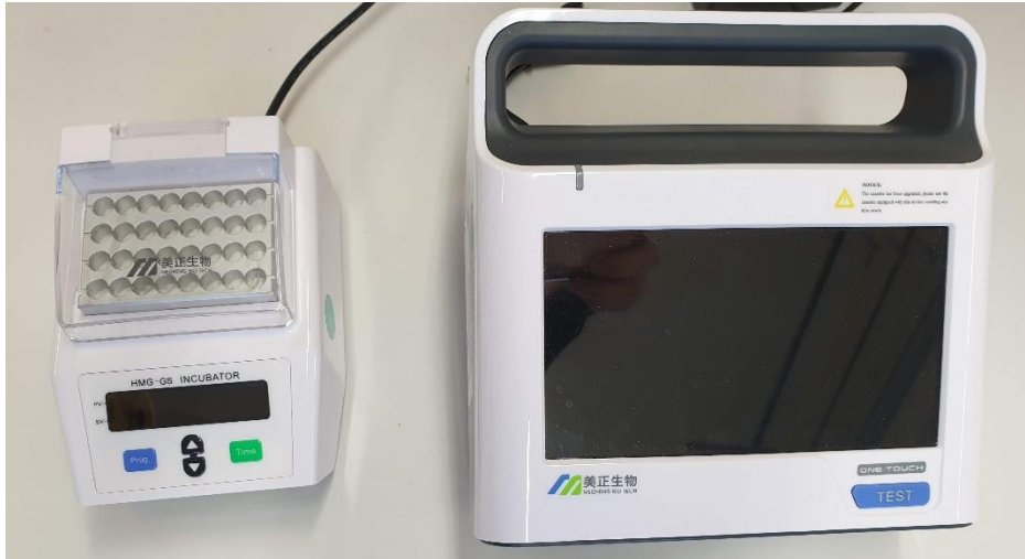
Fig. 2. HMG-GS Microwell Incubator and BMZ6000 Portable Strip Reader for instrumental reading of the color formation on the AnticFast® Beta-lactams Rapid Test Kit.
